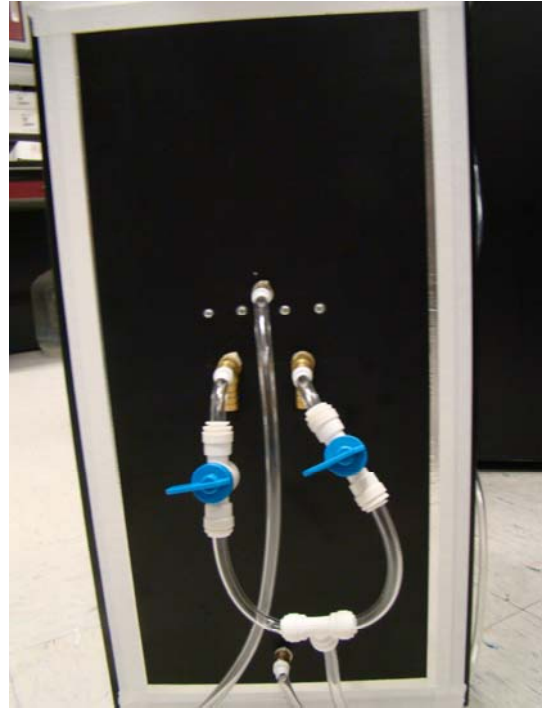
Figure 5. PVC Bypass Valves with "T" Connection
