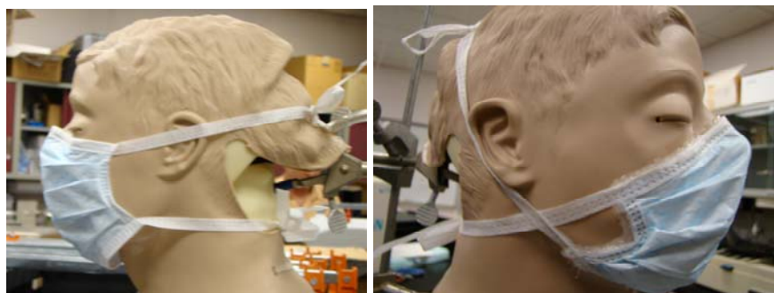
Figure 27. Unsealed mask under normal use Figure 28. Sealed mask with crossed straps
